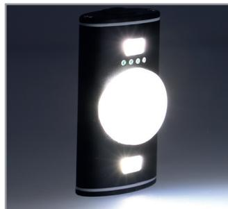
The NODUS lighting is designed in resin and aluminum with a silicone strap attachment that allows it to be easily positioned on all types of handlebars and seat posts. It is composed of a 0.5 Watt white LED which produces an intensity of 200 Lumens at the front and 25 Lumens at the rear. It works with a rechargeable lithium ion battery by USB cable. Using the light is very easy, just double click on the lens to turn it on and click once on the lens to change the different modes and turn it off.
