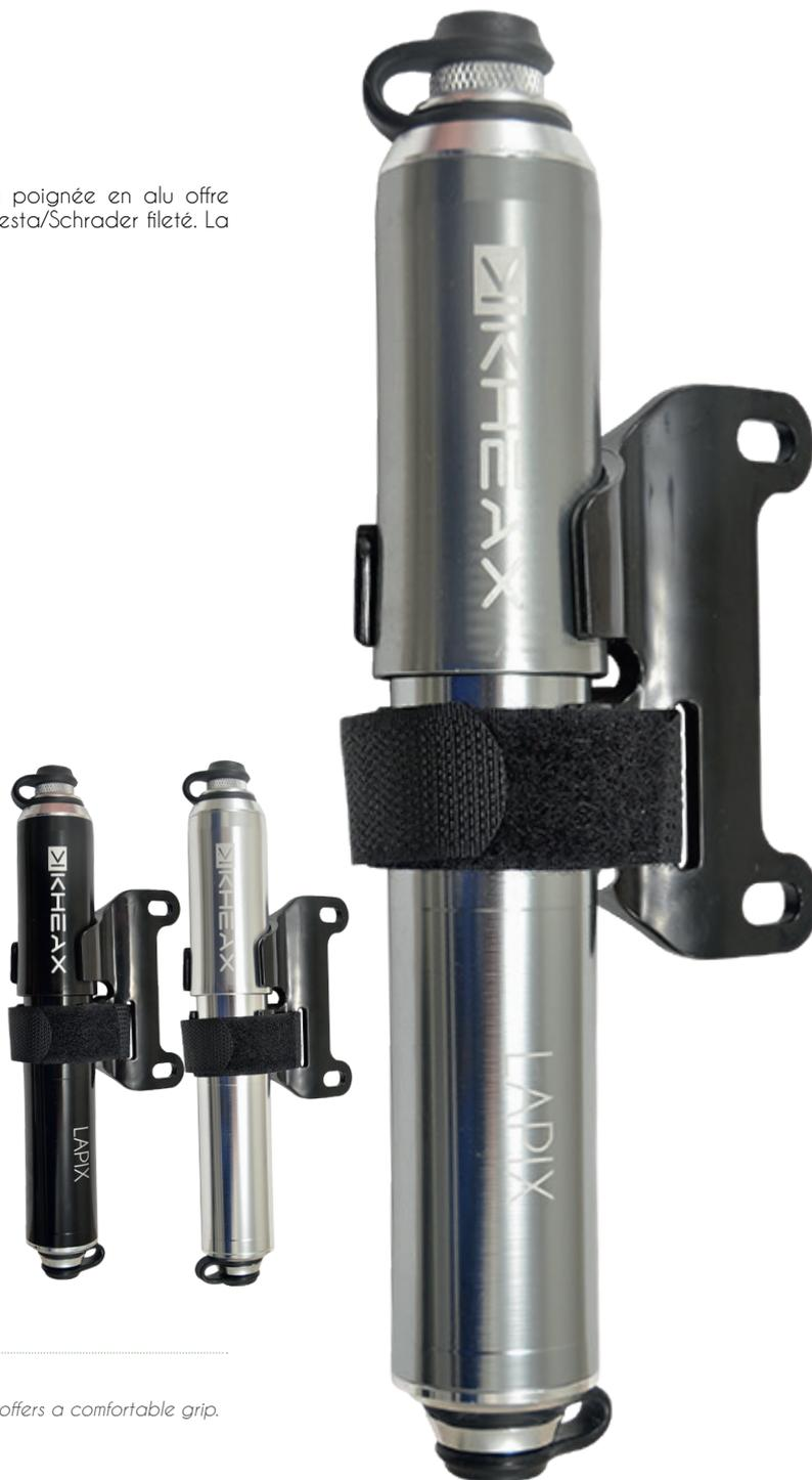
The LAPIX mini pump consists of a CNC aluminium body. The aluminium handle offers a comfortable grip. It is composed of a reversible Presta/Schrader threaded valve. The pump is delivered with a bottle cage mounting bracket. This product is available in 2 lengths (185 mm, 225 mm).
