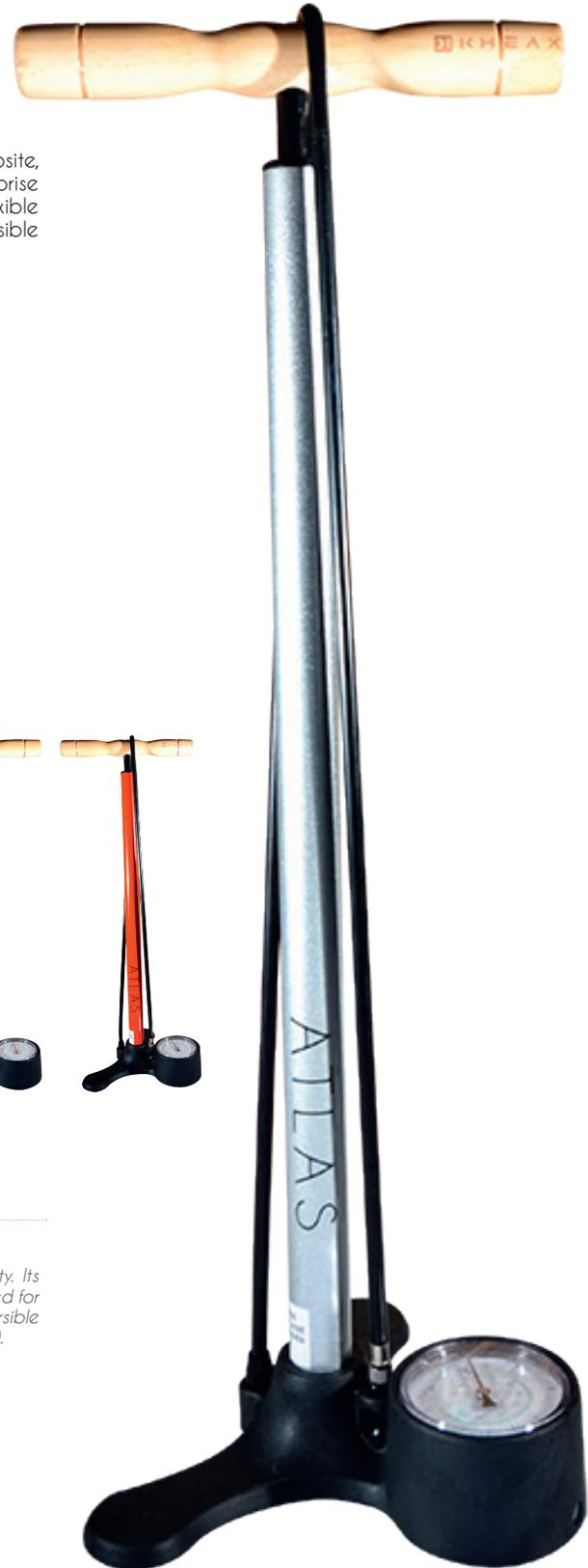
The ATLAS floor pump has a steel body and a composite base that provides a good stability. Its pressure gauge of 75 mm (2.95") diameter enables an easy reading. The wooden handle is designed for a comfortable grip. The pump hose is long (1230 mm) for easy inflating. It is composed of one reversible aluminium connector Presta/Schrader threaded valve and one universal kit (needle and cone tip). As an option, there is a bent connector (Presta/Schrader).
