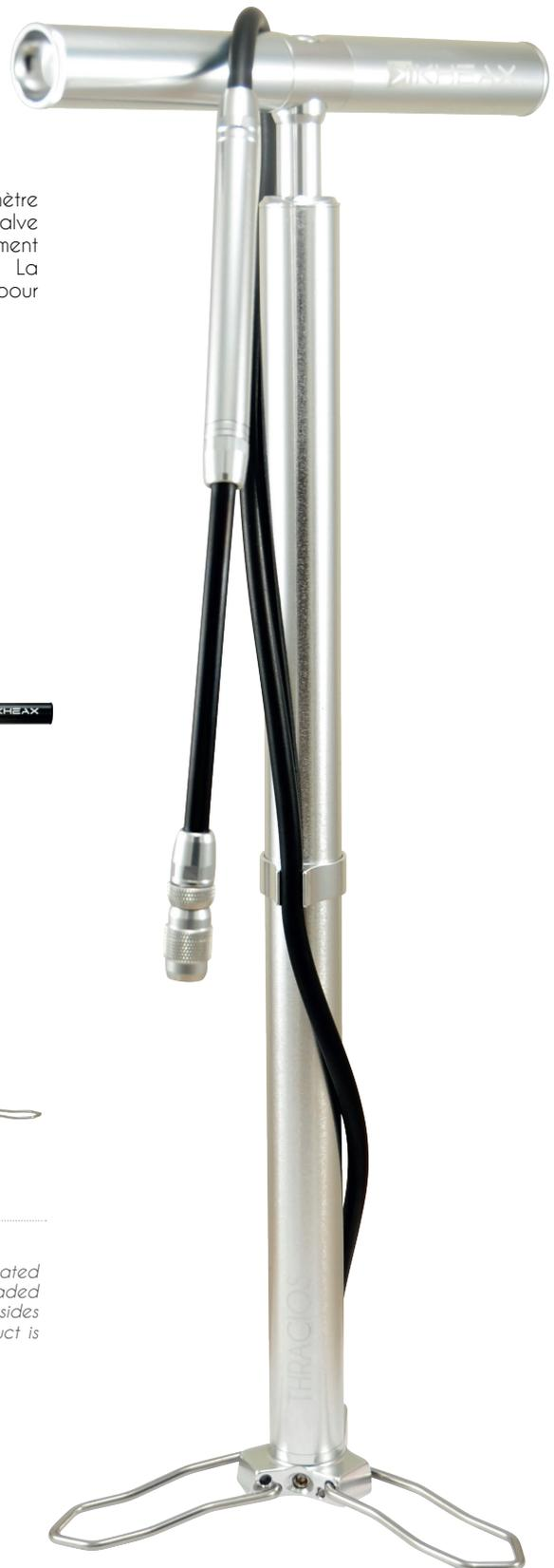
The TRAVEL THRACIOS floor pump consists of a CNC aluminium body. The pressure gauge is located on the pump hose. It is composed of a reversible aluminium CNC connector, Presta/Schrader, threaded valve. The CNC aluminium handle is removable and features storage space accessible by the sides (screwed aluminium caps). The pump folds up and is delivered with a carrying case. This product is especially designed to be handled easily and to be portable during your travels.
